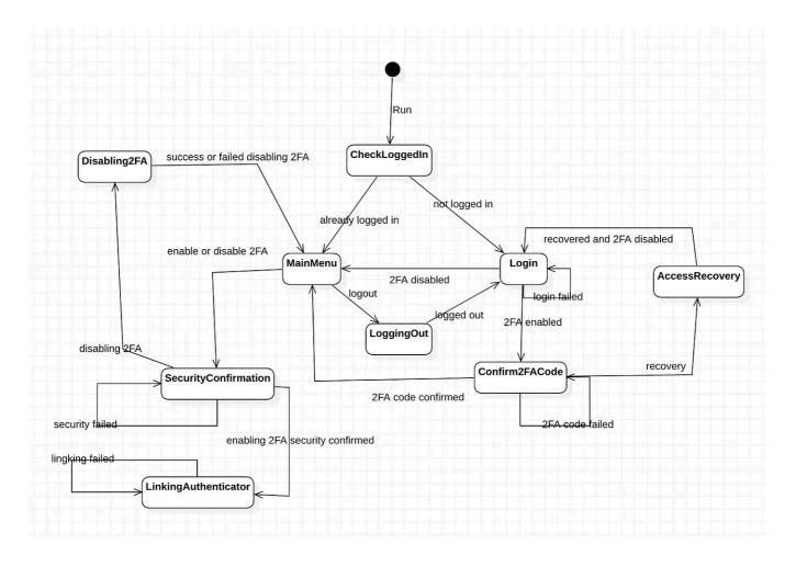
We refined the PRD into a statechart diagram so we can see the transitions from login to enabling the 2FA setting and seen the impact when logging out and reloggin in again, the sytem will ask for 2FA code. Also when disabling the 2FA the statechart reflect the impact when re-logging in again. After successfull recovery the system will ask the user to relogin again and the 2FA settings will be disabled so after successful login the system will not asked for 2FA code anymore.
